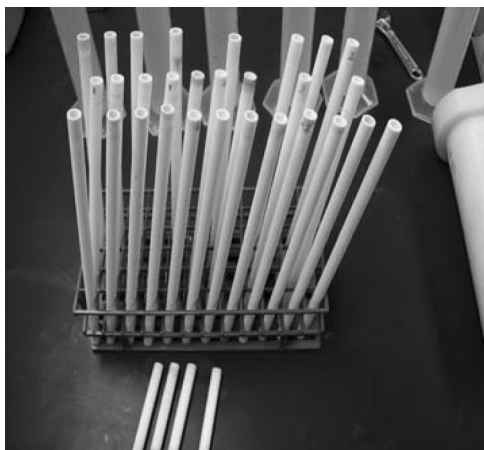
Figure 10. Tubular zeolite membranes on \alpha -alumina supports.
