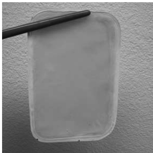
Figure 9. Compacted clay membrane formed by compacting under high pressure.
